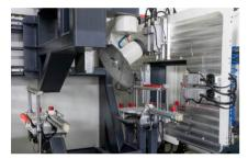
8 fan-cooled spindle motors which can operate at different angles, offer unlimited processing on 4 surfaces of the profile.
