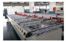
Conveyor with 4 profile feeding capacity ensures the machine to work in the most efficient way.
