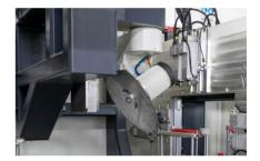
550 mm diameter saw that can cut at any angle between 0° and 180° thanks to its 5-axis movement capability, the saw allows cutting and end-milling operations of profiles up to 300 mm wide.
